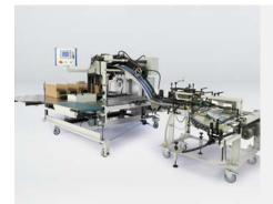
Omega Pack is a fully automated case packer to complement the high-speed carton production on Omega folder gluers. Omega Pack can pack up to 4 rows and 4 layers, requires a single operator and takes 10-15 minutes to make ready. It handles straightline
